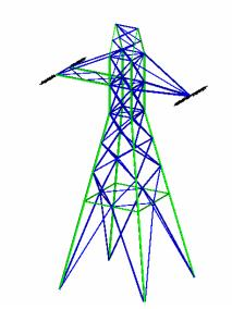
The figure at the left is a tower with the SET option for COLOR set to Element Type. BEAMS are green, TRUSS elements are blue.
