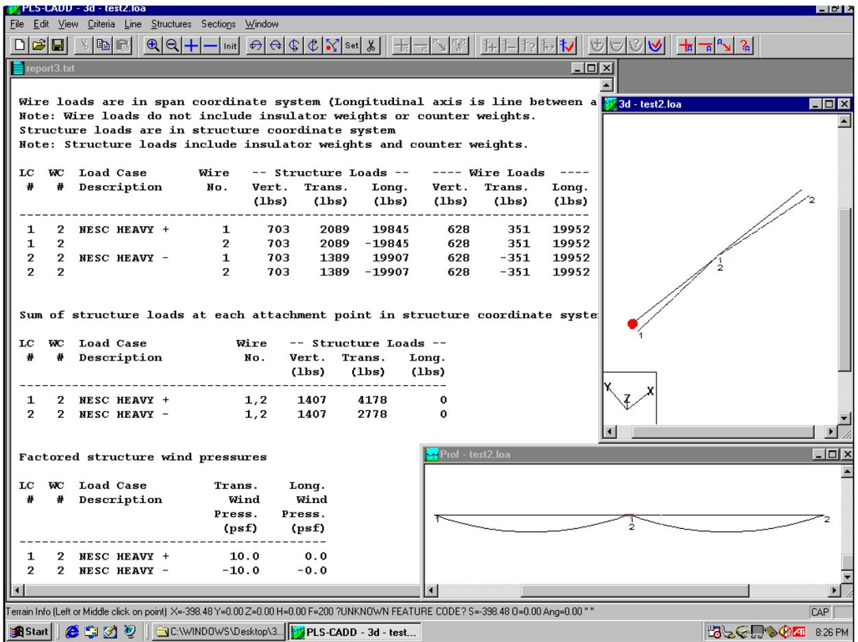
Fig. 15-6 Design loads for a simple two-wires model
