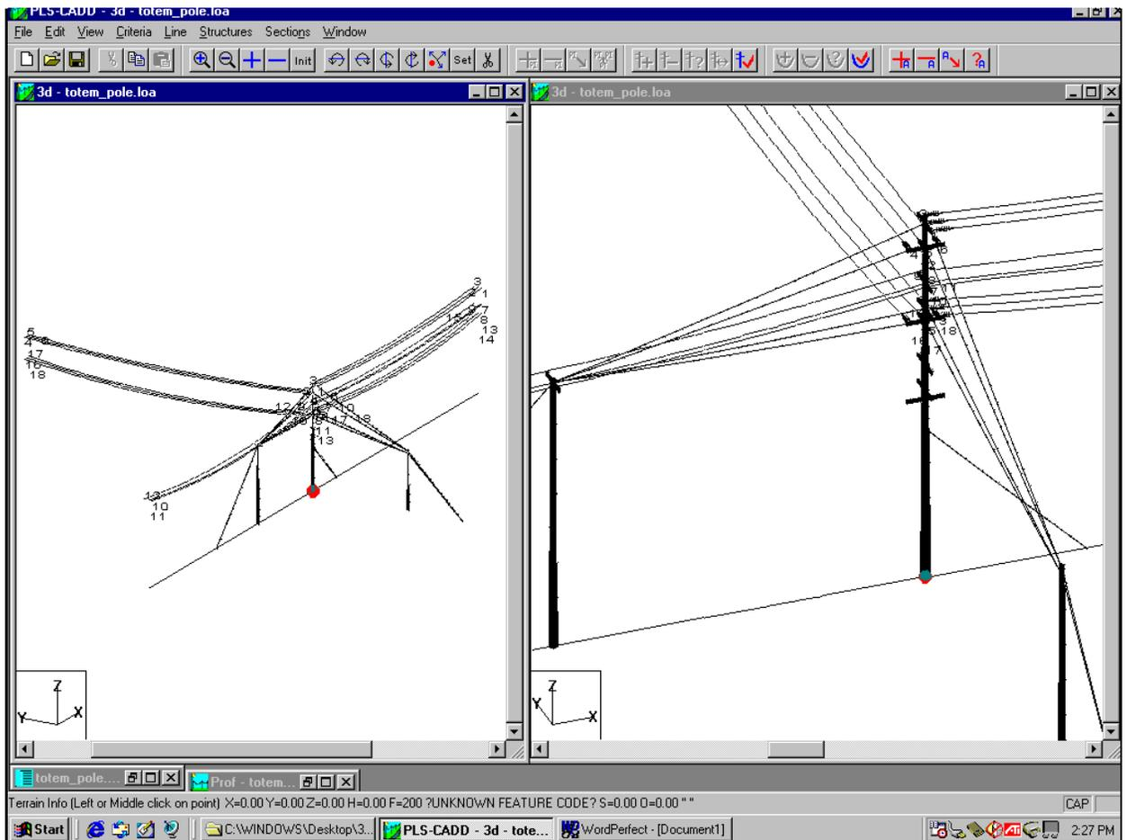
Fig. 15-1 Wood pole strung in PLS-CADD/ LITE
