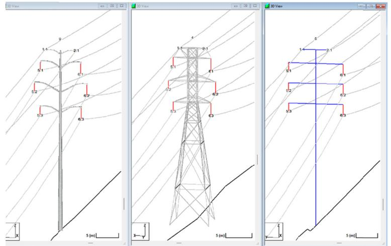
Figure 1 - Full structure models from PLS-POLE and TOWER compared to an Allowable Span file
