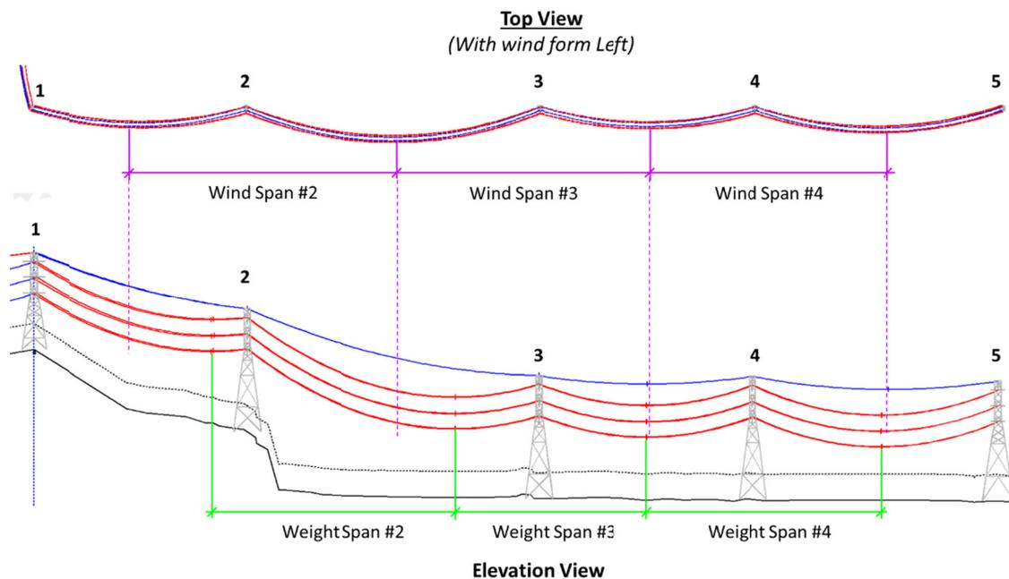
Figure 2 - Overview of Wind and Weight Spans
