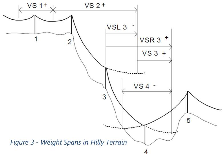
Figure 3 - Weight Spans in Hilly Terrain
