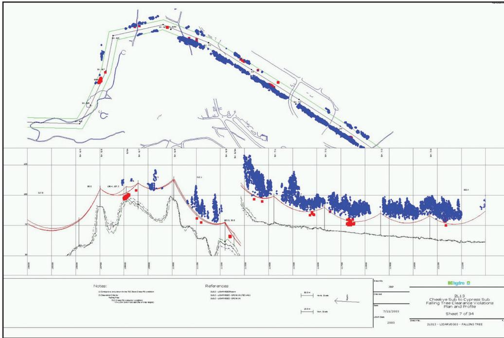
**Fig. 5. Plot of vegetation clearance violations produced directly from PLS-CADD.**
