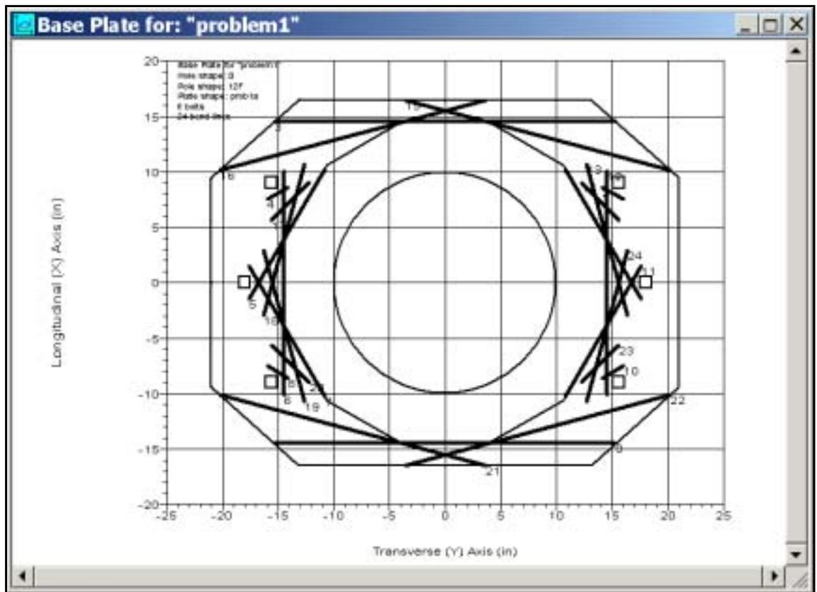
**Fig. 3.1.1-5 Base plate and effective bend lines**
