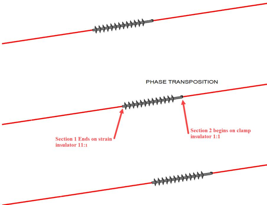
9. The next step is to add jumpers to model the phase transposition. First activate the jumpers within **Criteria/SAPS Finite Element Sag-Tension...**
