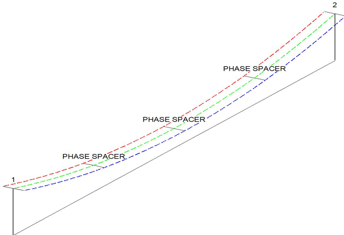
Phase spacers can be modeled in PLS-CADD using two methods. A simplistic approach is to add concentrated loads at the locations of the phase spacers to represent the weight and wind area of the phase spacers. This does not account for the interaction of the phases being tied together, but this simplification of the interphase spacers will be quicker to model, and allows the use of ruling span assumptions or L2 SAPS finite element analysis options.
