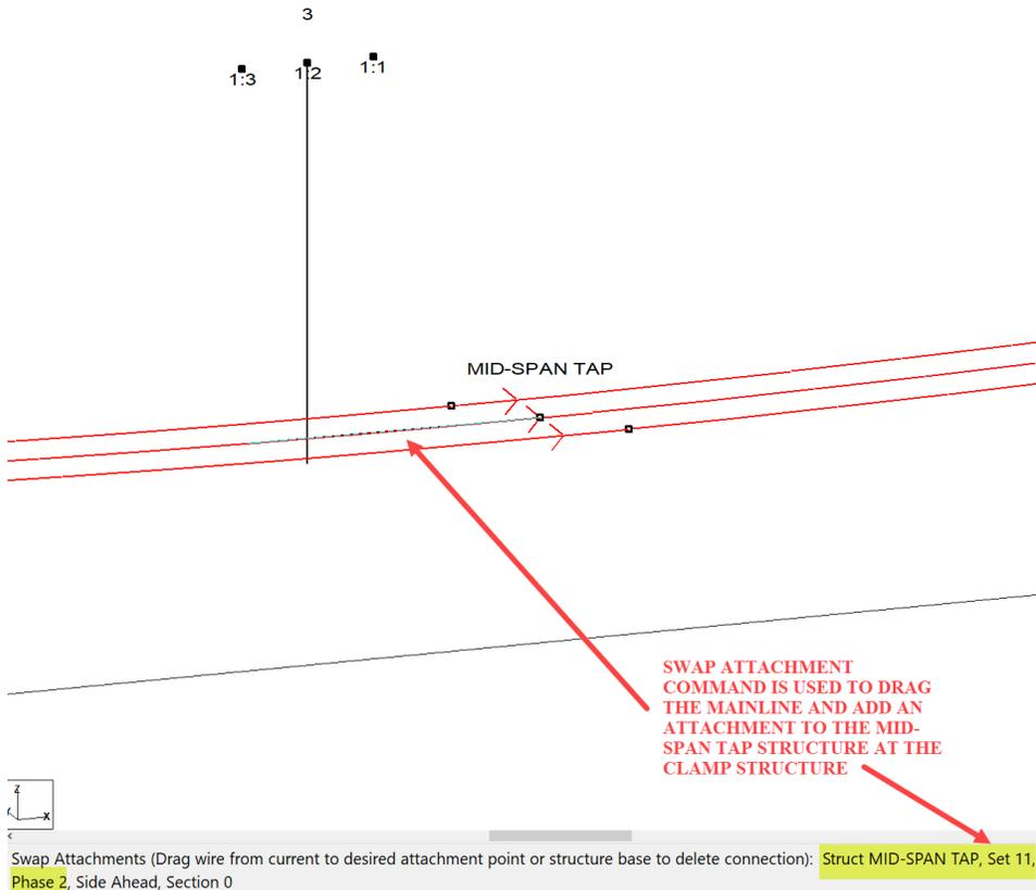
7. Then use the **Sections/ Add Graphical** to string between the mid-span structure and the structure the tap will connect to. This new section should attach to the strain insulators at the mid-span tap structure. When adding this tap the horizontal tension of the sections that make up the tap will need to be defined. PLS-CADD is not capable of stringing vertical wires, so if the tap is vertical a small offset is needed so the wire attachments are not in a vertical plane.
