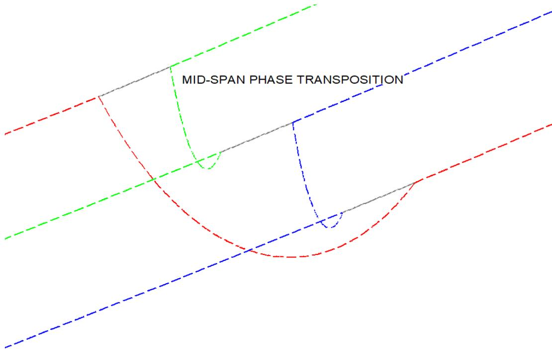
Phase transpositions can be modeled in PLS-CADD with the use of PLS-POLE or TOWER structures and jumpers in PLS-CADD. Modeling these transpositions requires SAPS for the finite element capabilities to model jumpers and Level 4 SAPS analysis to attach insulators to structure files with free joints. To model a phase transposition you can use the following method:
