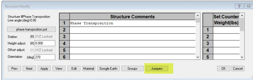
11. Finally the circuits and phases can be updated. To do so the graphical methods with the menu command **Sections/Electric/Edit Circuit Connection** or tabular method **Sections/Electric/Define Circuits and Phases/Table...** can be used to update the circuit and phase. The jumpers will help link the phase labels between the back and ahead spans at the phase transposition structure.
