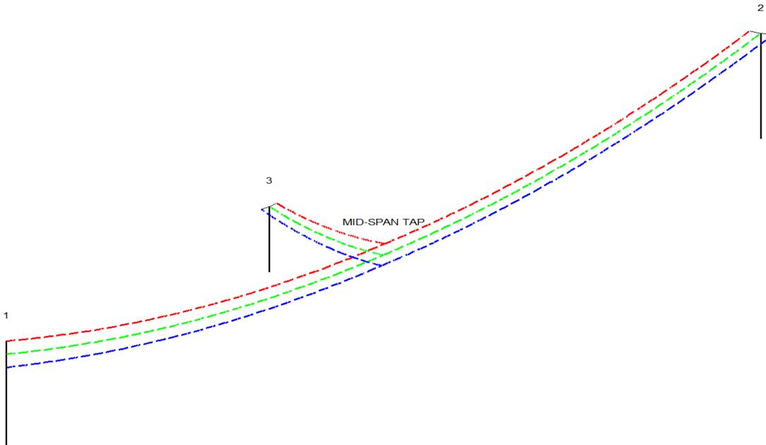
Mid-Span taps (Flying taps) are possible in PLS-CADD with the use of PLS-POLE or TOWER structures and Level 4 SAPS analysis. The procedure below describes how Mid-Span tap structures can be created and spotted in a
