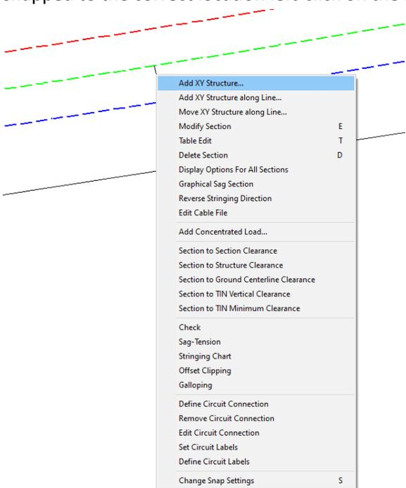
It is also possible to add this structure as an alignment based structure but the user will have to adjust the height of the structure so that is attached at the proper height of the wires.
