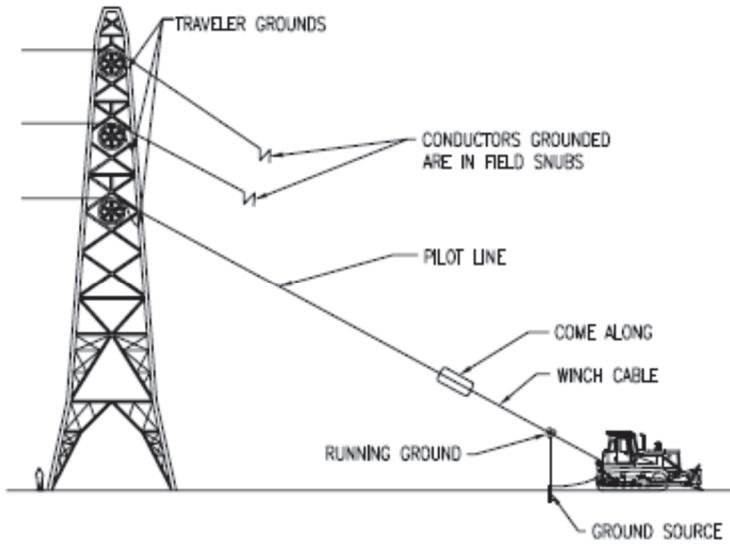
During the pulling and sagging/tensioning operations, the deadend structures at the end of the tension section(s) will experience these snub loadings. Due to the extreme tensions and loads that deadend structures are designed for under extreme meteorological events, they are usually adequate for the everyday tensions experienced during the construction operation. However, it is obviously a good idea to verify this, especially for lattice towers
