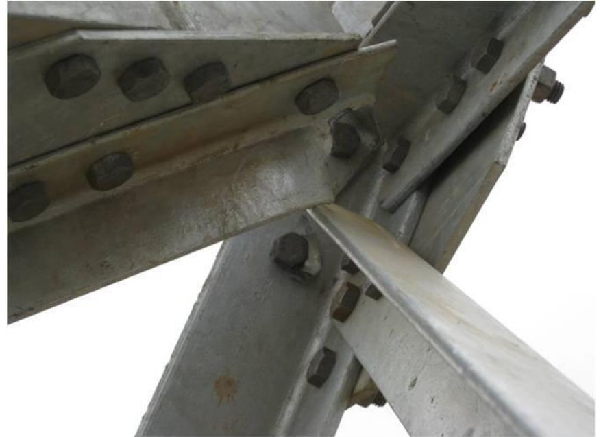
Incorrectly detailed bolt pattern failed during testing of 10 degree angle structure
