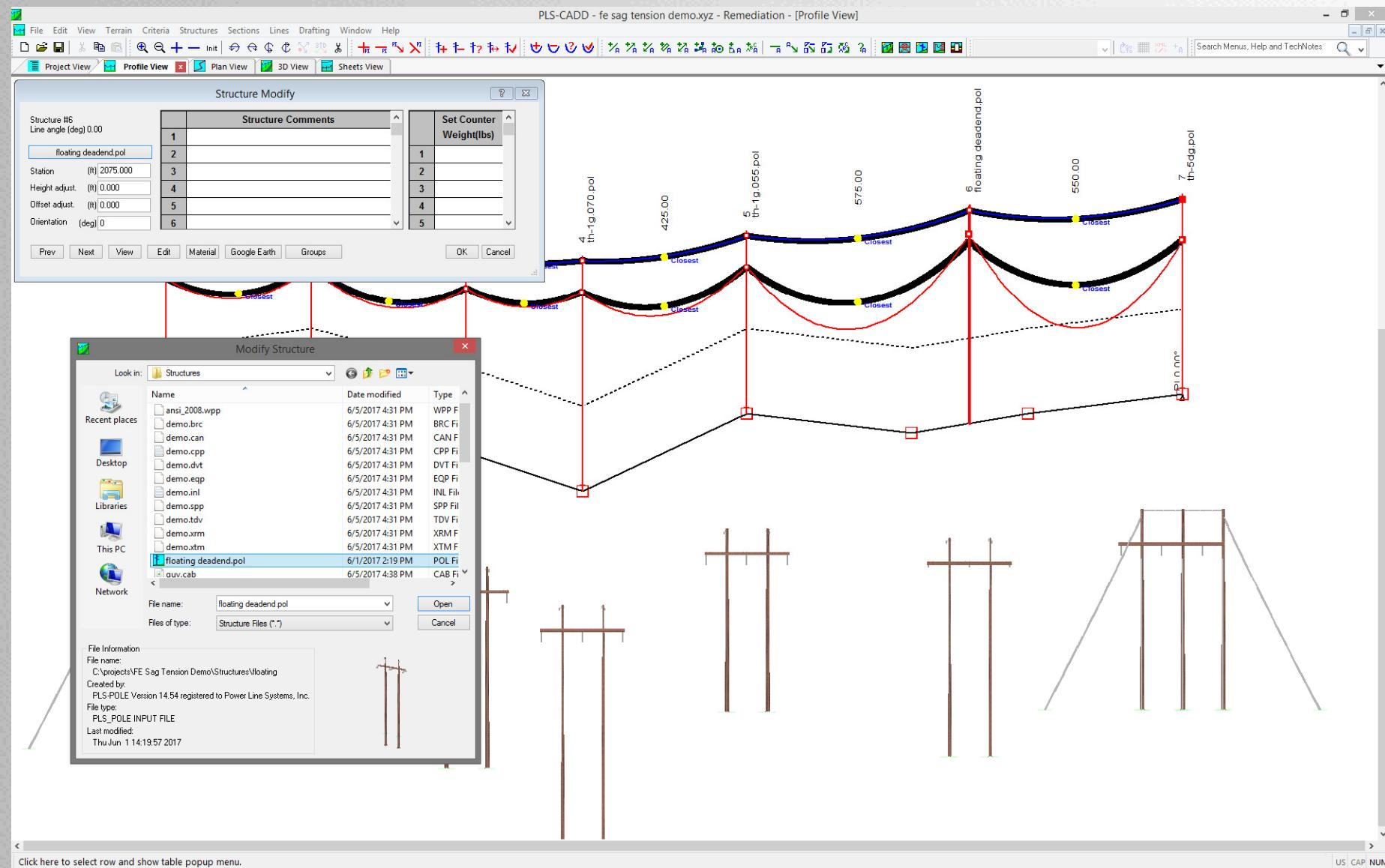
\*Note: Extra sag in wires in spans adjacent to floating dead end caused by inserting strain insulators into the span
