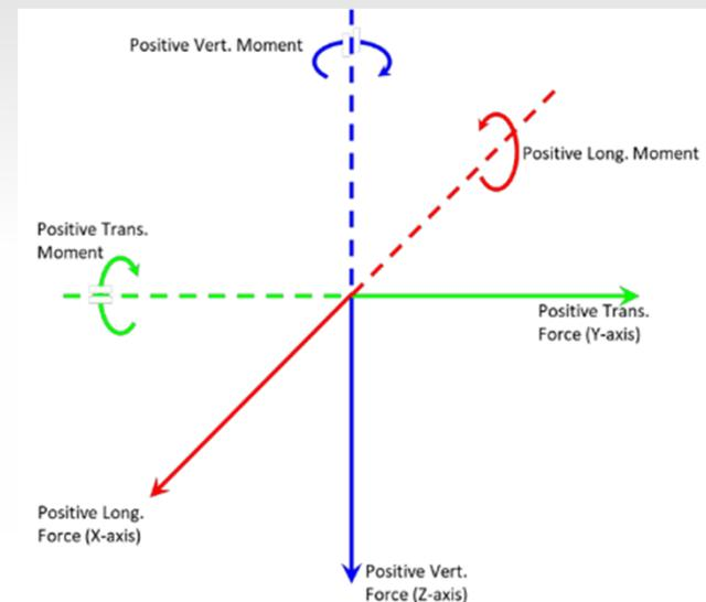
Figure 3.7-1 CAN Coordinate System
