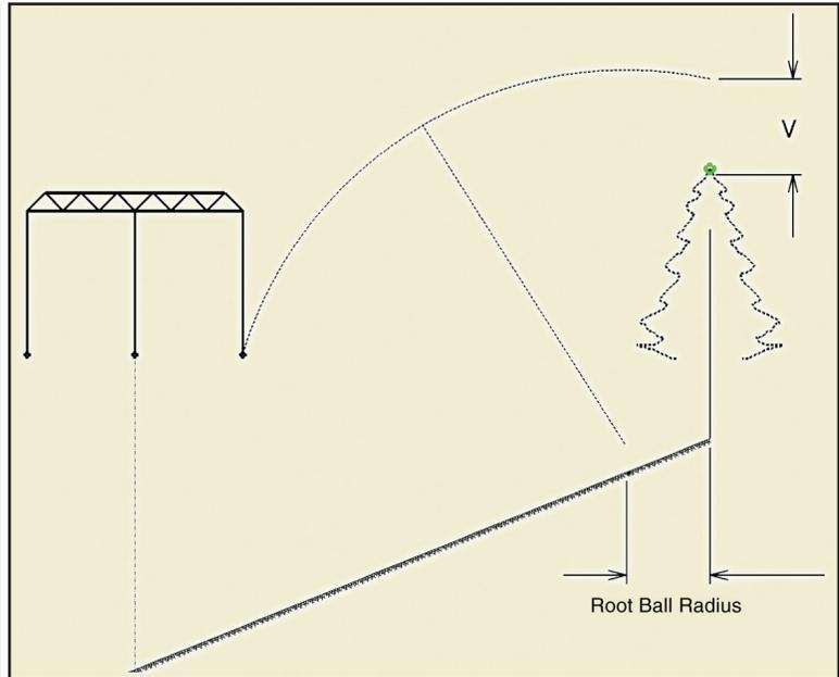
Fig. 4. Falling tree clearance requirements.
